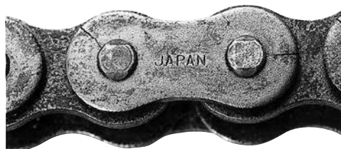
Hydrogen embrittlement cracking
